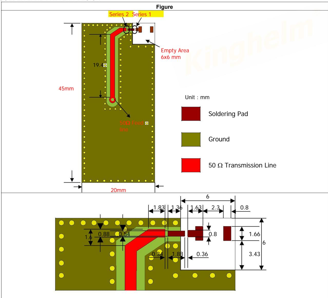
Antenna on Test Board ( Thickness 1.2mm)
